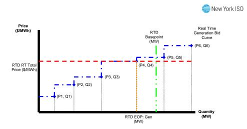
In the diagram below, the RTD interval LBMP intersects the given Generation Bid block on a horizontal line and the Generator was Base Pointed below the given Generation Bid block. In this case, the Generator's EOP is equal to the lower Generation Block MW (i.e.,  $Q_3$ ) of the block where the RTD interval LBMP intersects the Generation Bid.
